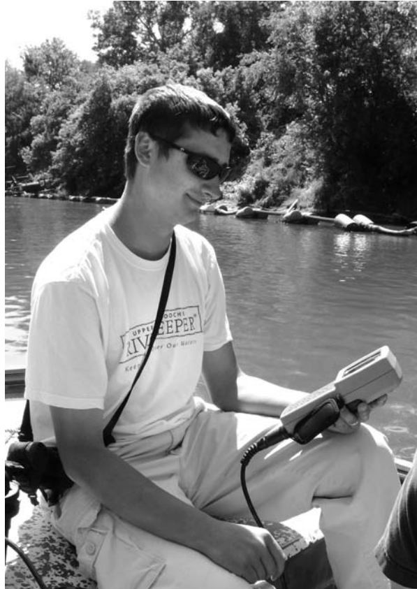
Jason Ulseth, UCR Watershed Protection Specialist, measures dissolved oxygen downstream of Peachtree Creek aboard our patrol boat.
